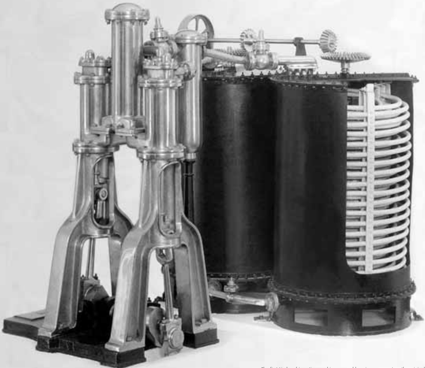
The first Linde refrigeration machine ever sold, an improvement on the original model from 1873, started up in 1877 at the Dreher Brewery in Trieste (now Italy).
